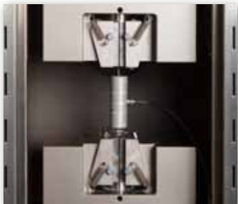
Alignment Meets Nadcap AC7101 and AC7122 Specifications
