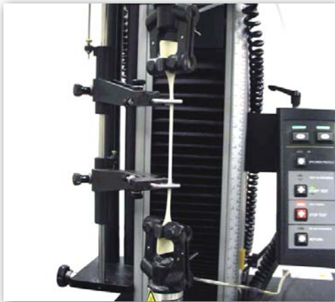
Long-travel extensometer used for rubber tensile elongation test to ASTM D412 and ISO 37
