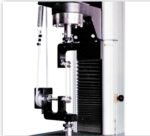
Elastomeric o-ring test to ASTM D1414
