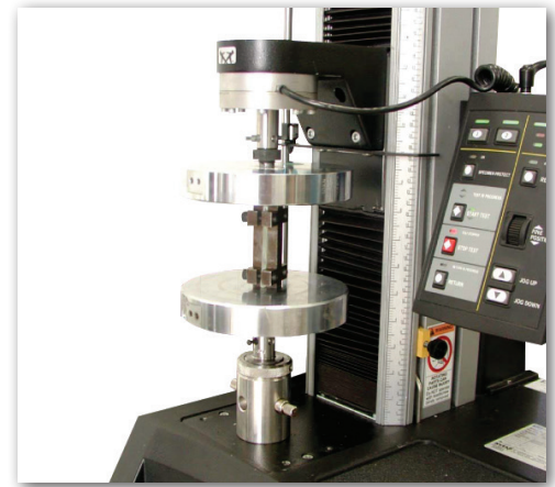
Test configuration for in-plane shear strength of reinforced plastics according to ASTM D 3846
